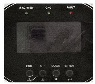
Left (green light):Solid light - Utility bypass; Flashinverter mode;
